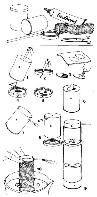
This very efficient pump is quite easy to make. It requires two film-roll plastic cases, 15-cm of old cycle tube, an old refill or a short thick straw (like the one found in tetra packs of fruit juices) and a rubber-based adhesive like *Fevibond* or *Vamicol*.
