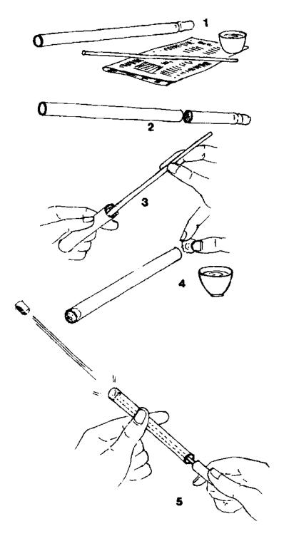
Take a 30-cm long piece of bamboo with an internal bore of 8-10 mm.
