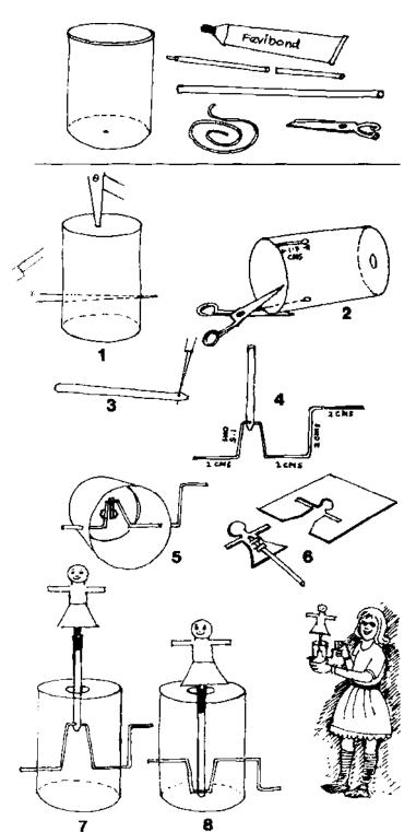
As you rotate the handle of this little machine, the doll on top jumps up and down.
